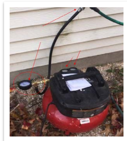
Air compressor with gauges connected to system in order to confirm system is holding pressure.
