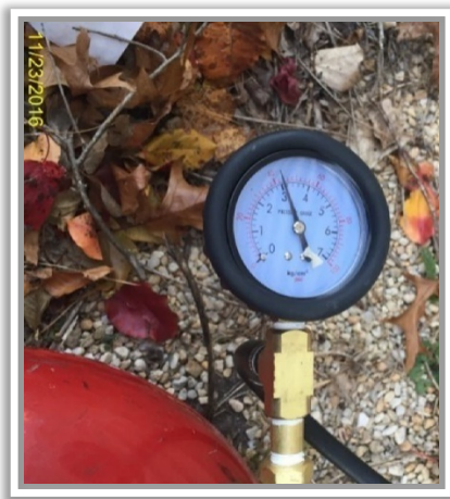
Air compressor with gauges connected to system in order to confirm system is holding pressure.
